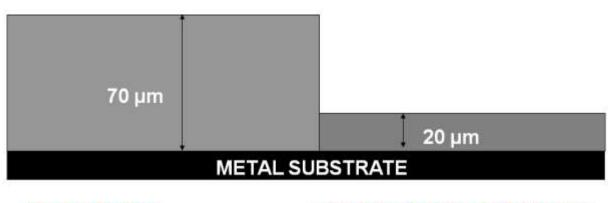
Standart Coating Specific Gravity : 1.65 gr/cm<sup>3</sup> Coating efficiency : 8.66 m<sup>2</sup>/kg
